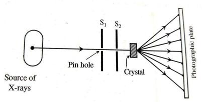
**Fig. Experimental Arrangement of Laue Method**
