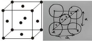
In Face Centered Cubic Lattice 8 atoms occupy 8 corners of unit cell and 6 atoms occupy 6 faces. Consider a face of FCC lattice.
