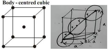
In Body Centered Cubic Lattice 8 atoms occupy 8 corners of unit cell and 1atom at the center. Consider the corner atoms and center atom.
