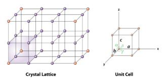
The lines drawn parallel to the lines of intersection of any three faces of the unit cell that don't lie in the same plane are called crystallographic axes. Three translational vectors a, b and c lie along the crystallographic axes. These three vectors are the intercepts that define the dimensions of unit cell are known as primitives.
