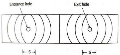
the film is exposed for a few hours in order to obtain arcs of sufficiently high intensity. It is removed from the camera and developed. The circular arcs are observed on the film as shown in figure. From the figure, the angle  $\theta$  corresponding to a particular pair of arcs is related to the distance S between the arcs.
